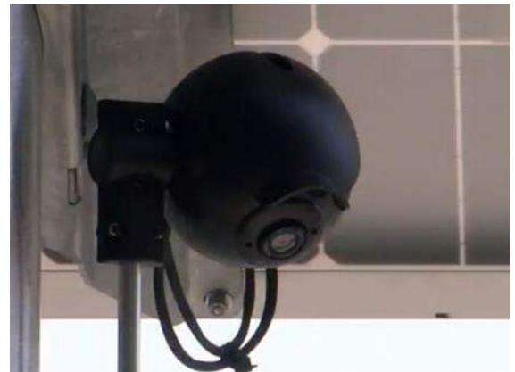
► New thermal sensor installed at the Trail Crossing that automatically activates the flashing lights for bicyclists crossing Skinner Boulevard.
