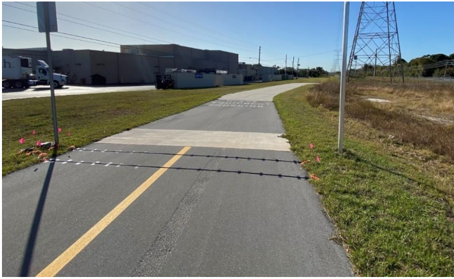
Figure 3-3: Pneumatic Counters on the Pinellas Trail and Sunset Point Road On Sunset Point Road both EB and WB
