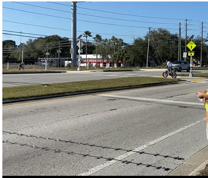
Figure 3-3: Pneumatic Counters on the Pinellas Trail and Sunset Point Road On Sunset Point Road both EB and WB
