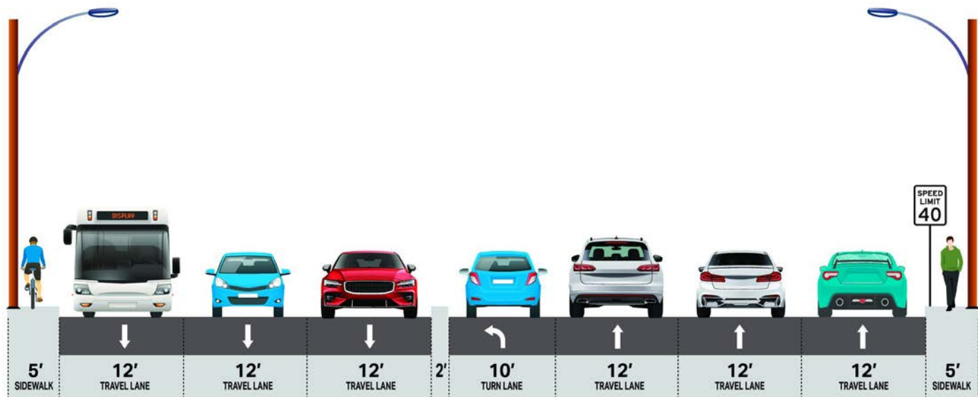
Typical Section: Six-Lane Divided Arterial, C4-Urban General Context Classification, 40 MPH Posted Speed
