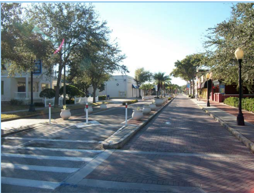
This roadway in Tarpon Springs includes components of a complete street, providing sidewalks and a buffered multi-use trail facility that enhances safety and accommodates more than just automobile traffic.
