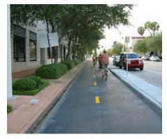
**Separated Bikeway** (Cycle Track / Protected Bikeway)
